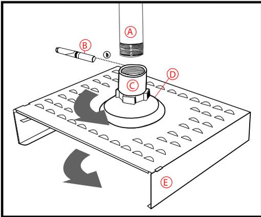
1. Apply the Pipe Adhesive (B) to the inside of the Coupler (C) at the top for approximately 3 threads down.
