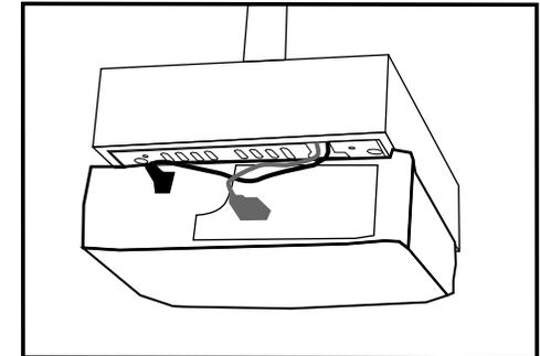
2. Slide the Grid Plate (F) (or Media Shelf) in while guiding the cables into a slot located in the back of the Grid Plate (or Media Shelf).
