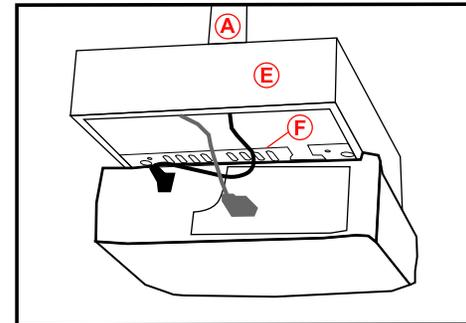
1. Before completely closing the mount, route the cables from the Pipe (A) out along the back of the Receiver Tray (E).
