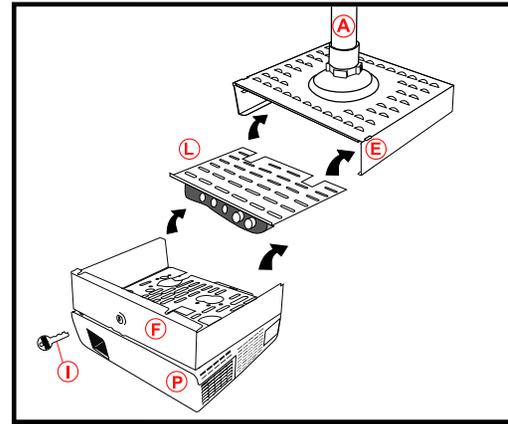
1. After the Receiver Tray (E) has been attached to the Pipe (A), the Media Tray (L) is in place and the Projector (P) has been attached to the Grid Plate (F), slide the Grid Plate 3 inches into the Receiver Tray.
