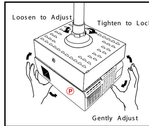
1. Turn ring counter clockwise to loosen mount.
