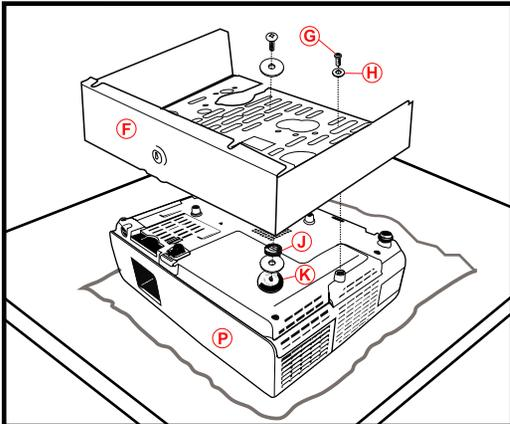
1. Place the Projector (P) upside down on a soft cloth and remove or lower the feet as much as possible.
